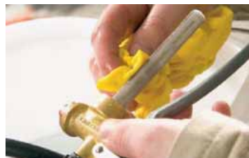
Clean filters of the vaccine equipment after use
