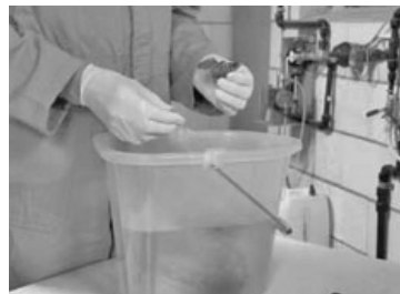
Dissolving Vac-Safe in a bucket for automatic dosing system
